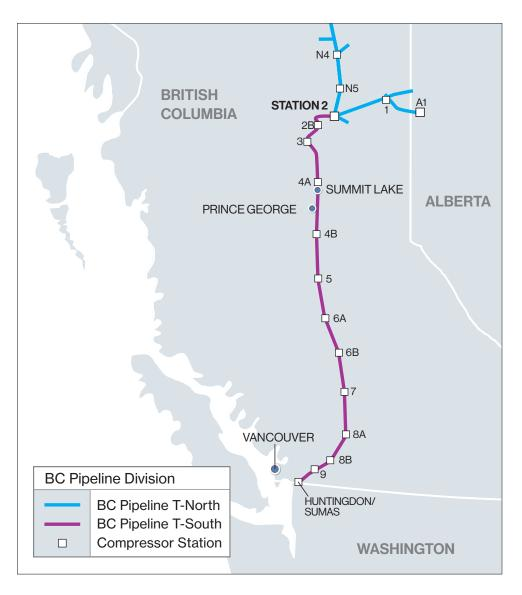
50 miles, apart) compress and push the gas to maintain its velocity and pressure as it travels through the system.
